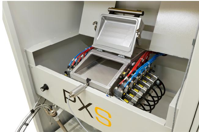
The optional ultrasound sieve can be fully integrated into the fluid tank.
