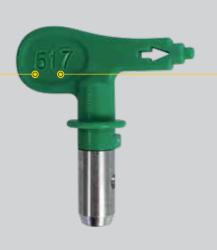
**Orifice diameter:** The orafice diameter (in this case, 0.017 inch) determines the flow volume and thus the amount of paint applied.
