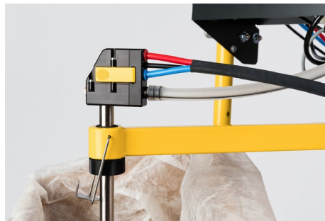
Right: Quick-Link injector with Quick-Link coupling for fast cleaning and color change
