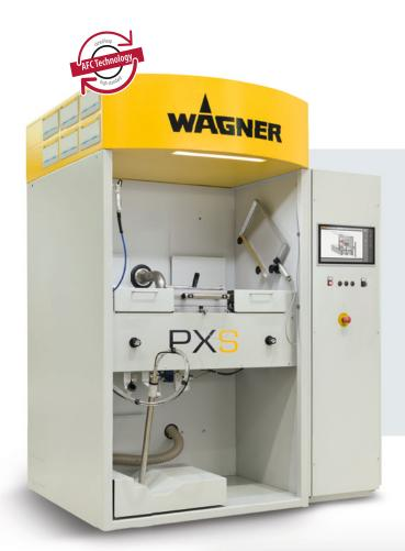
The PXS powder center is not only the central powder supply element, it is also the centerpiece of the entire coating system.
