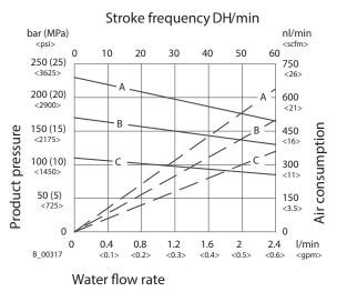
A = 8 bar (0.8 MPa; 116 psi) air pressure B = 6 bar; 0.6 MPa; 87 psi air pressure C = 4 bar; 0.4 MPa; 58 psi air pressure B 0390
