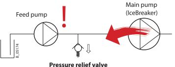
→ The pressure-relief valve must be cleaned regularly and after each activation: Flush with solvent.
