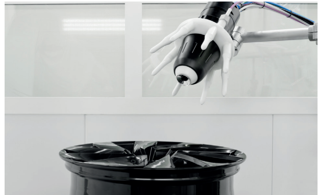
High-speed rotation atomizer with external charging
