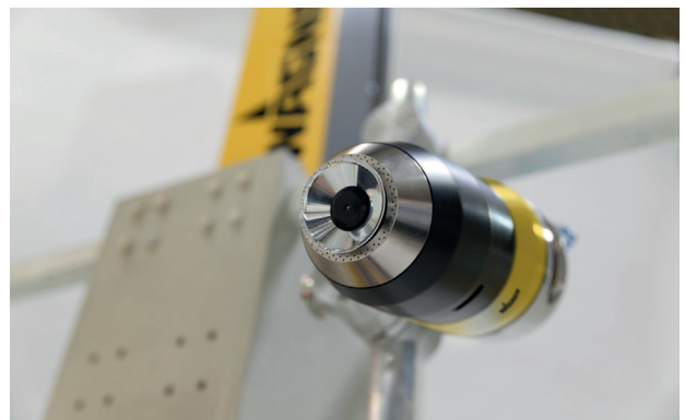
High-speed rotation atomizer with internal charging
