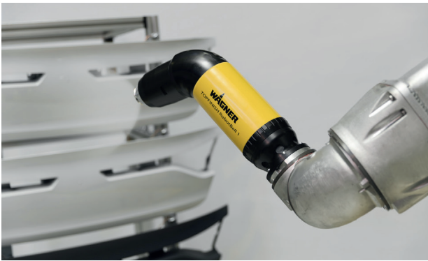
High-speed rotation atomizer mounted on a robot arm
