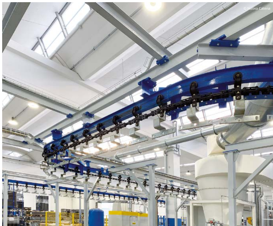
Overview of the conveyor supplied by Nuova Catena and a detail of the Morris-type chain.
