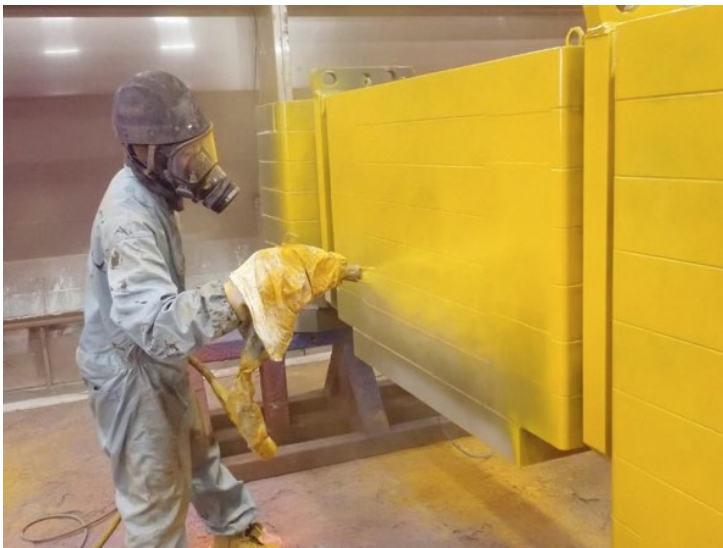
Electrostatic coating of crane components with the GM 5000EAC manual gun
