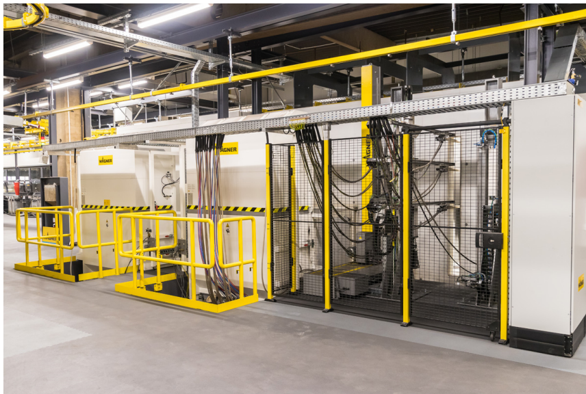
Every booth has compact, modular filter systems with low ceilings and recovery facilities.
