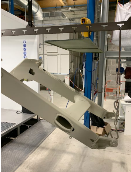
Components for agricultural machinery during the coating process
