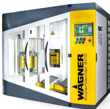
SuperCenter EVO for fast color changes with a high degree of automation
