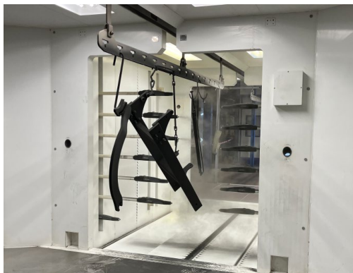
3D powder coating of workpieces in the S-Cube color booth
