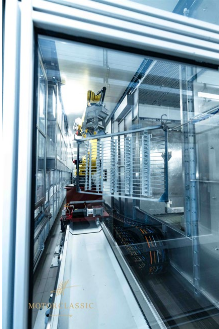
Left: One of the transfer robots transports the coating frames between the system units Right: Parts of exterior mirrors for the automotive industry
