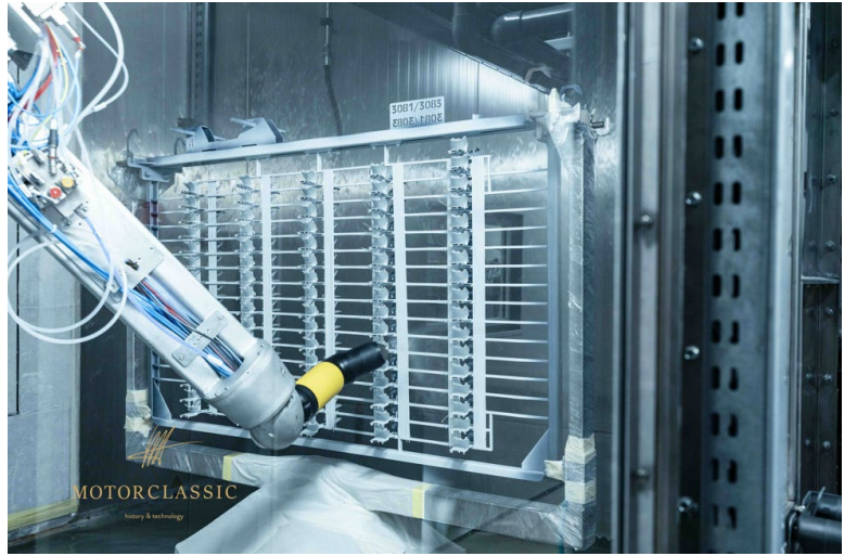
The TOPFINISH RobotBell 1 high-speed rotation atomizer applies the clear coat
