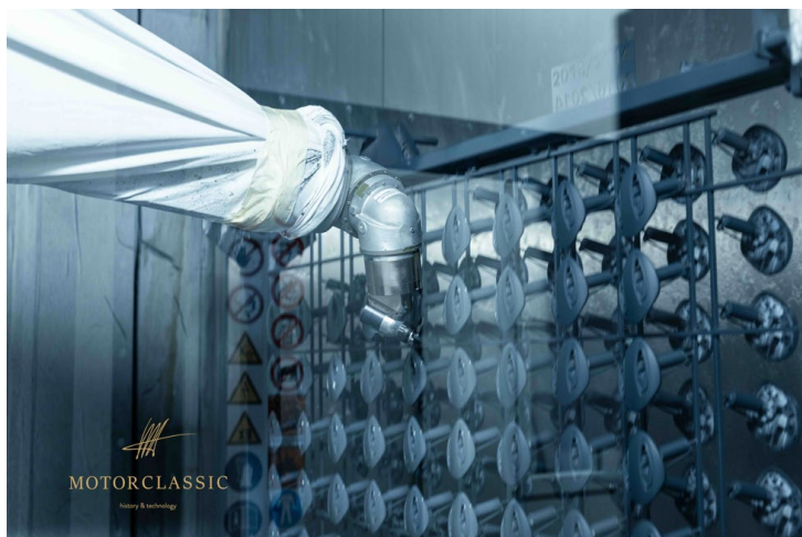
Airspray gun GA 1900 for paint application with extremely fine atomization
