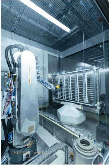
The TOPFINISH RobotBell 1 high-speed rotation atomizer applies the clear coat
