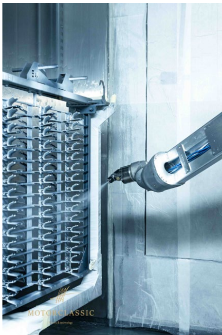
Airspray gun GA 1900 for paint application with extremely fine atomization
