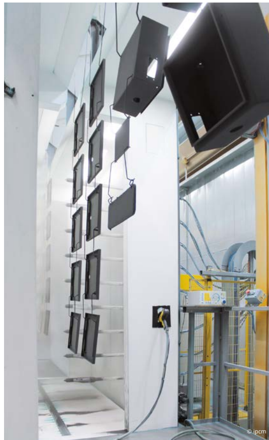
Single-colour paint application in the booth installed by Wagner in 2008 (left photo) and a booth applying different colours.
