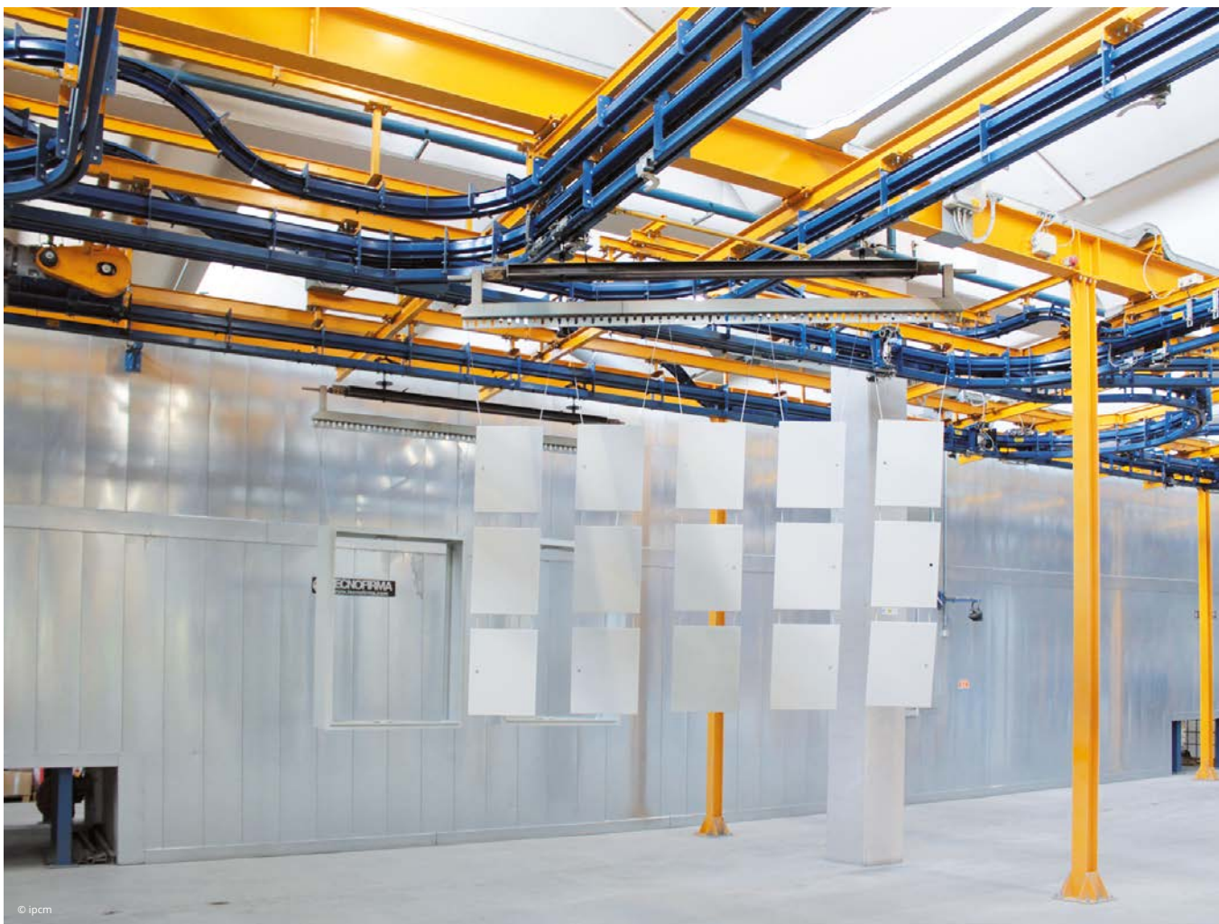
The conveyor takes the coated parts to the curing oven.
