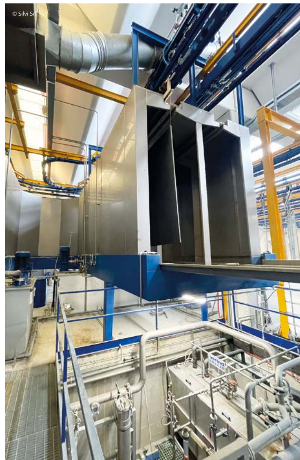
The cataphoresis tank and the double-pass through UF cleaning tunnel made in 316 stainless steel.
