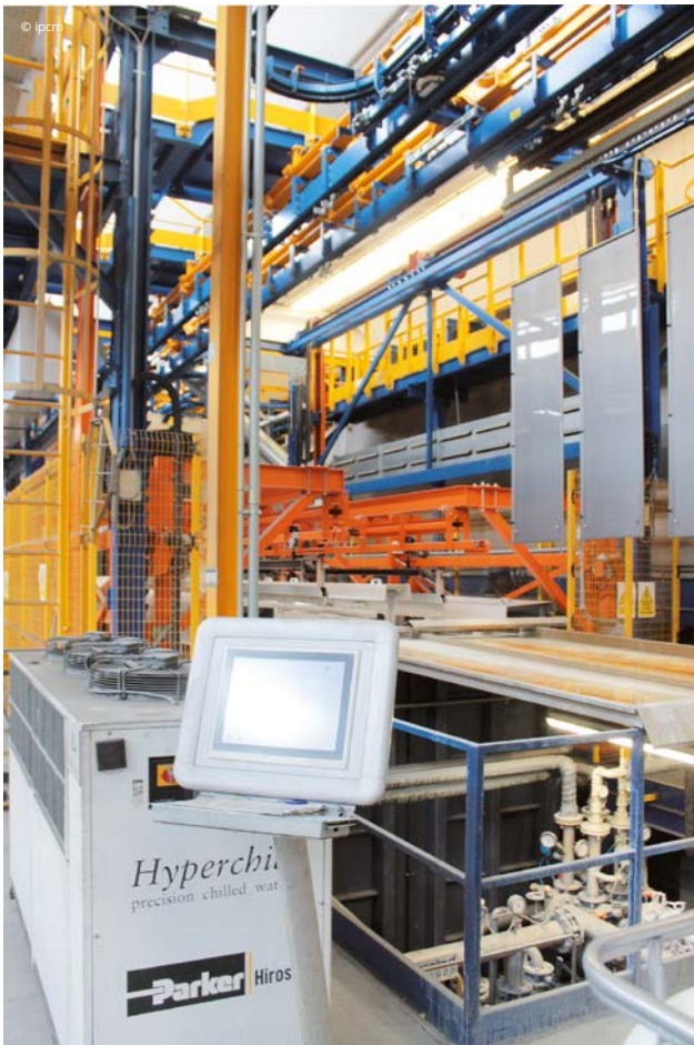
The PLC controlling the cataphoresis process, interconnected with the company's management system and the drying oven from Tecnofirma SpA.
