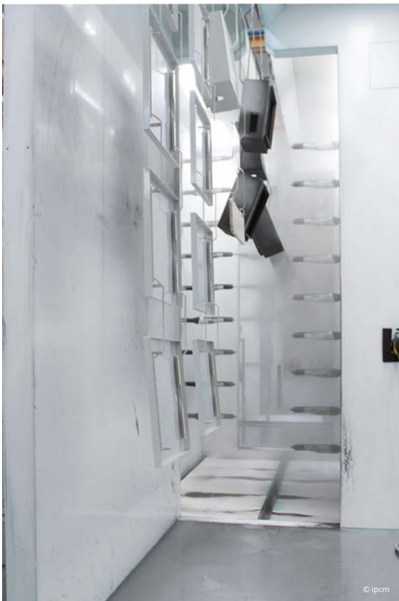
Single-colour paint application in the booth installed by Wagner in 2008 (left photo) and a booth applying different colours.
