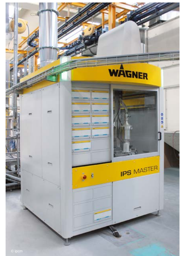
The IPS system managing the multi-colour booth: the Smart Boxer can accommodate two boxes at a time and automatically switch from one to the other for continuous-flow powder feeding. On the right, the IPS module for multi-colour powder management.
