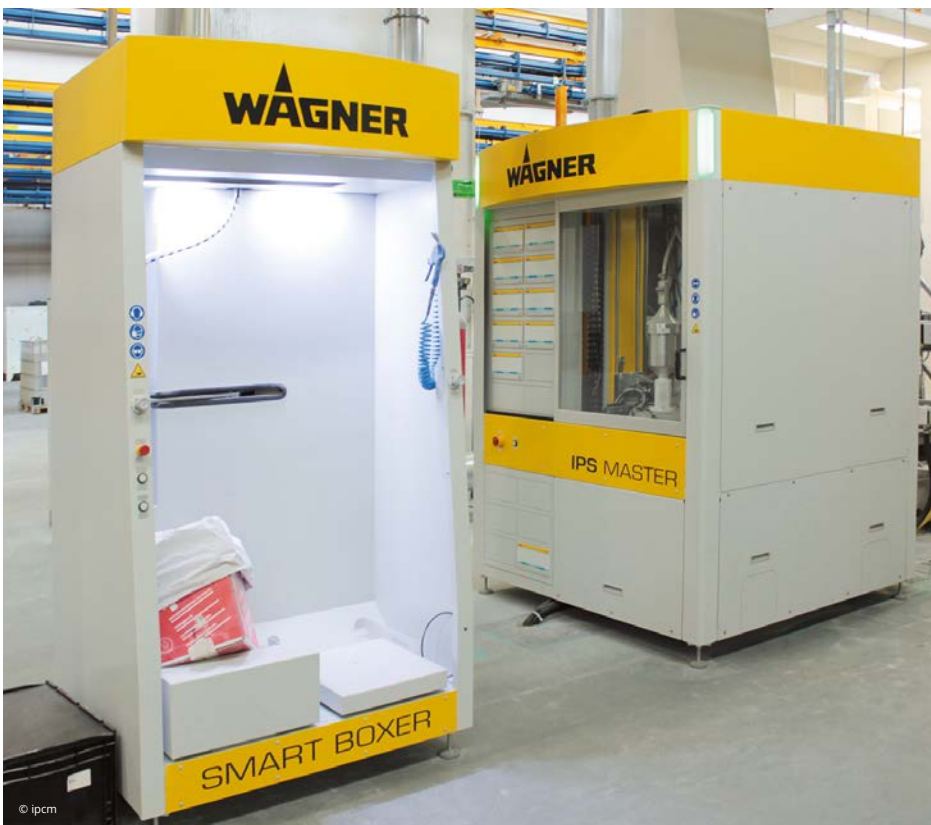
The IPS system managing the multi-colour booth: the Smart Boxer can accommodate two boxes at a time and automatically switch from one to the other for continuous-flow powder feeding. On the right, the IPS module for multi-colour powder management.
