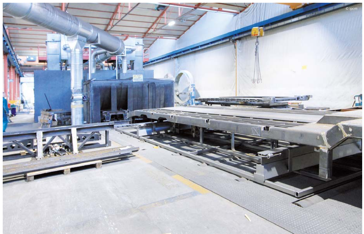
The shot blasting area within the coating department. In the background on the right, the prototype roll handler used to move the chassis.
