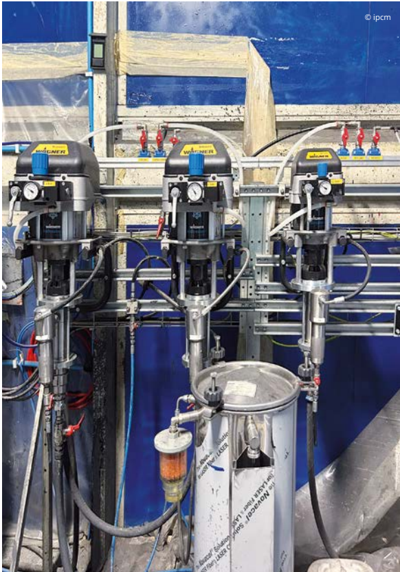
Both systems are equipped with Leopard 35-70 high-pressure piston pumps, with a volumetric flow rate of 70 cm 3 /DH for the catalyst and the paint product.
