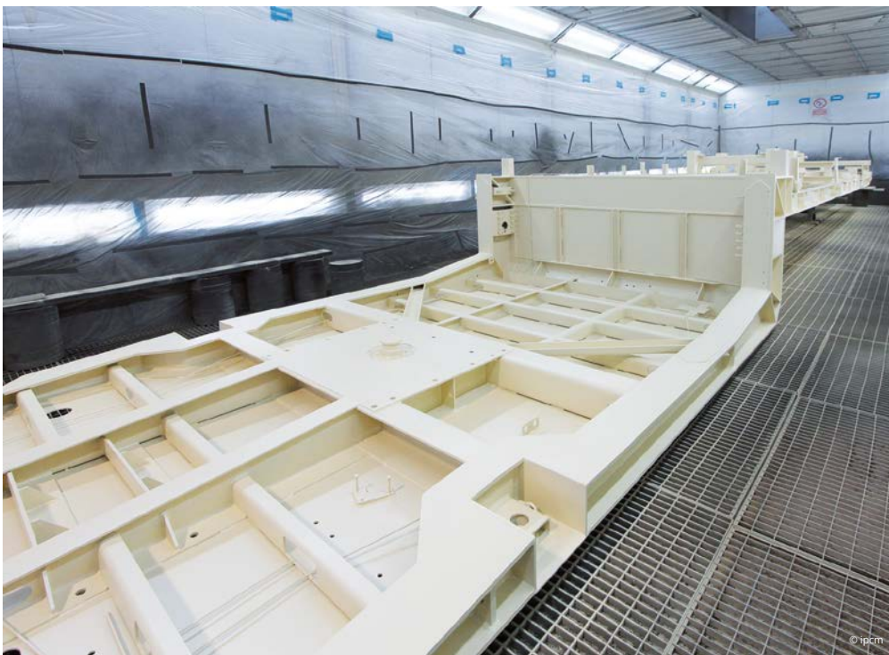
Inside one of the 2 coating booths, which can accommodate medium-sized parts measuring up to 13.5 x 2.5 m.
