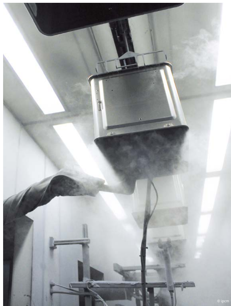
In the foreground, the 6-axis robot coating the 'ceiling' of an oven cavity.
