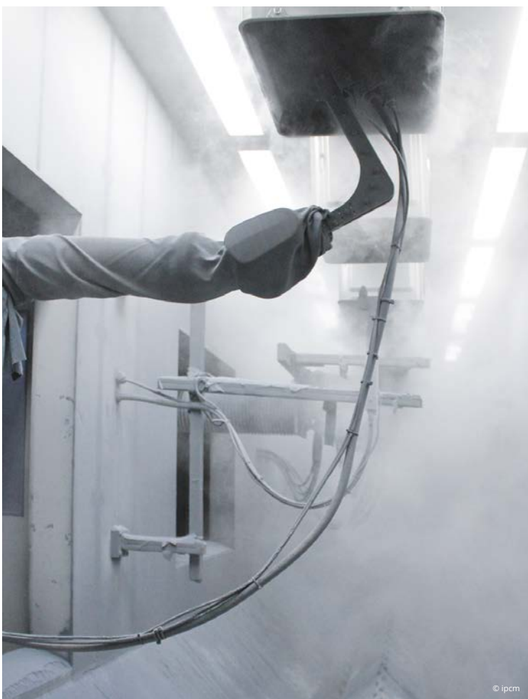
The inside of the Wagner enamelling booth for cavities.
