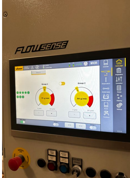
PXS powder center with Flowsense technology for the digital measurement of the powder output
