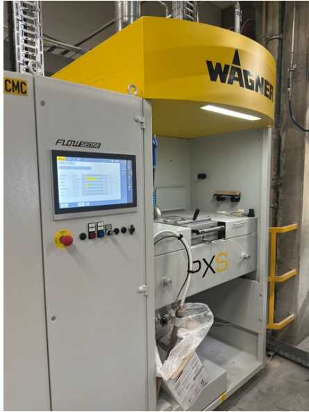
PXS powder center with Flowsense technology for the digital measurement of the powder output
