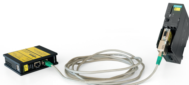
Connection to PLC with MPI interface MPI Ethernet adapter required for LAN connection
