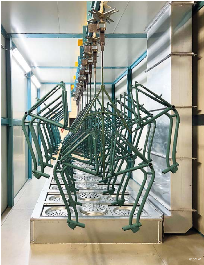
After powder application, the components enter the curing oven for about 24 minutes at 180 °C and finally reach the cooling tunnel.
