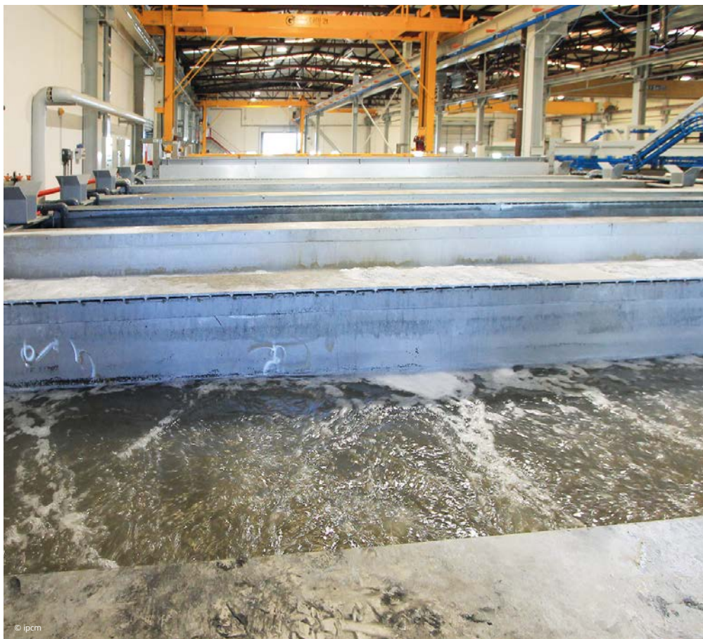
A detail of one of the tanks for the pre-treatment of aluminium products.
