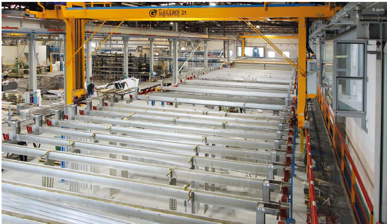
The storage buffer in the anodising and pre-treatment department.
