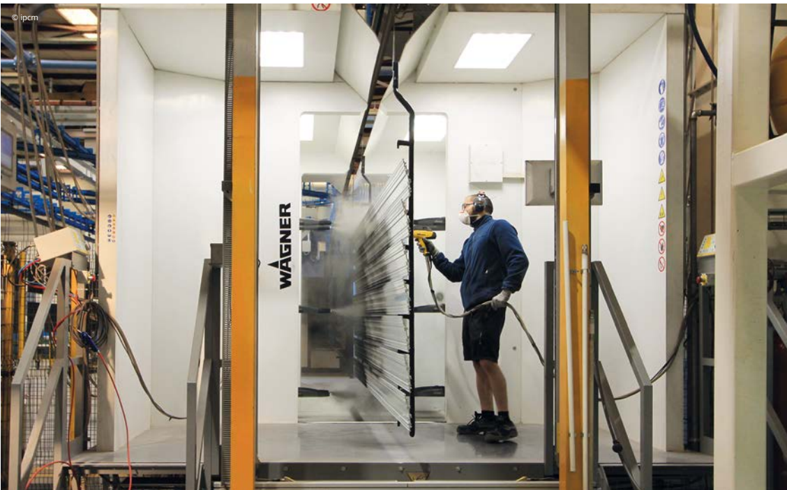
Manual pre-retouching is one of the strategic steps of Oxicolor's coating process. The PLC controlling the manual touch-up phase (on the right) is located close to the operator's workstation.
