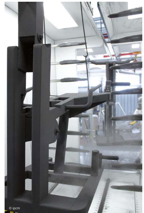
With the Smart Feeding Technology, the powder is fed through a pressure container and an electronically controlled dosing valve and generates a soft cloud with little overspray.
