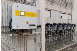
The 2K COMFORT automatic mixing and dosing systems have each been equipped with one additional special paint pump for Liebherr. It mixes minimal quantities of the subsequent top coat with the primer in order to optimize it and make it more brilliant.
