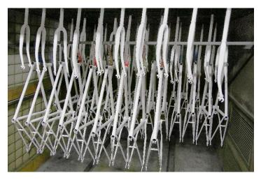
The particles adhere to the frame during powder coating due to the electrostatic charge. The paint is then cured into the bicycle frame in an oven or dryer.
