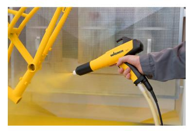
Krüger has opted for a new powder coating system. A manual system is used for this, which is particularly suitable for small batch sizes and frequent color changes. Among others, the PEM-X1 manual gun is used. (Picture source: J. Wagner GmbH)
