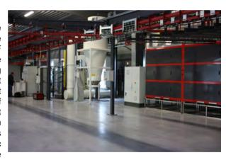
Secondly, Kempa wanted to make production more efficient and above all save working time. "Using the new system, two employees create several kitchens each day. Powder coating is more than twice as fast as liquid coating and we can immediately further process the workpieces without any drying time," says Filip Laureyssen. The procedure improves quality at the same time: In just a single, seamless work step, a coat is applied that is not only cheaper, but also more resistant and durable.
