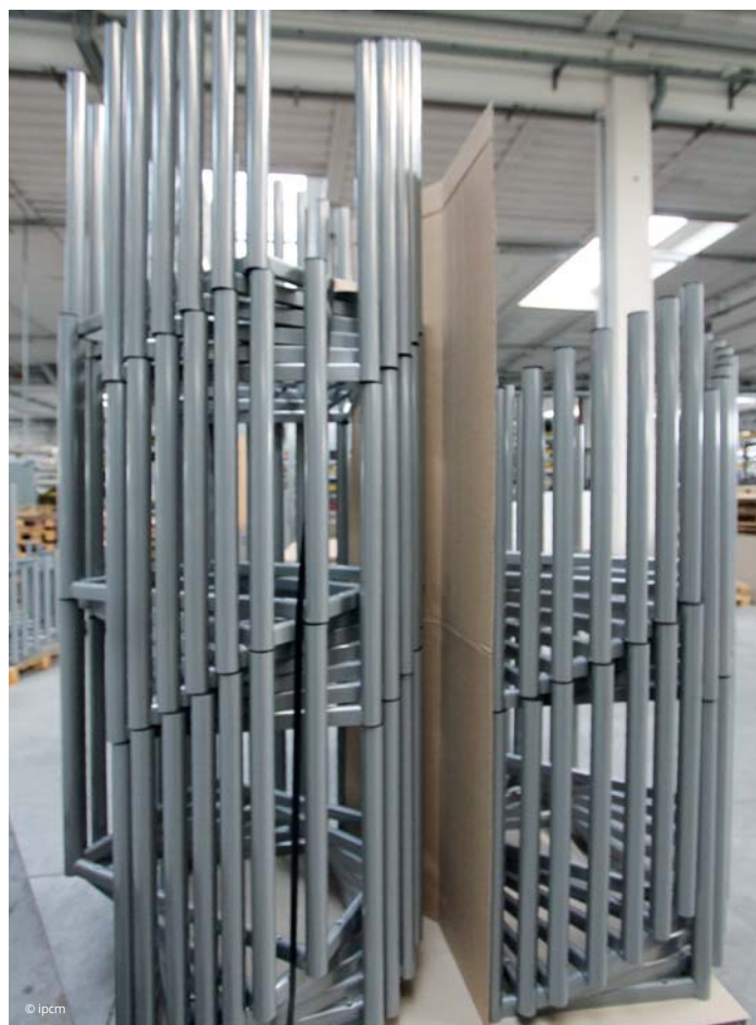
Metal structures for school desks, after machining and before coating.
