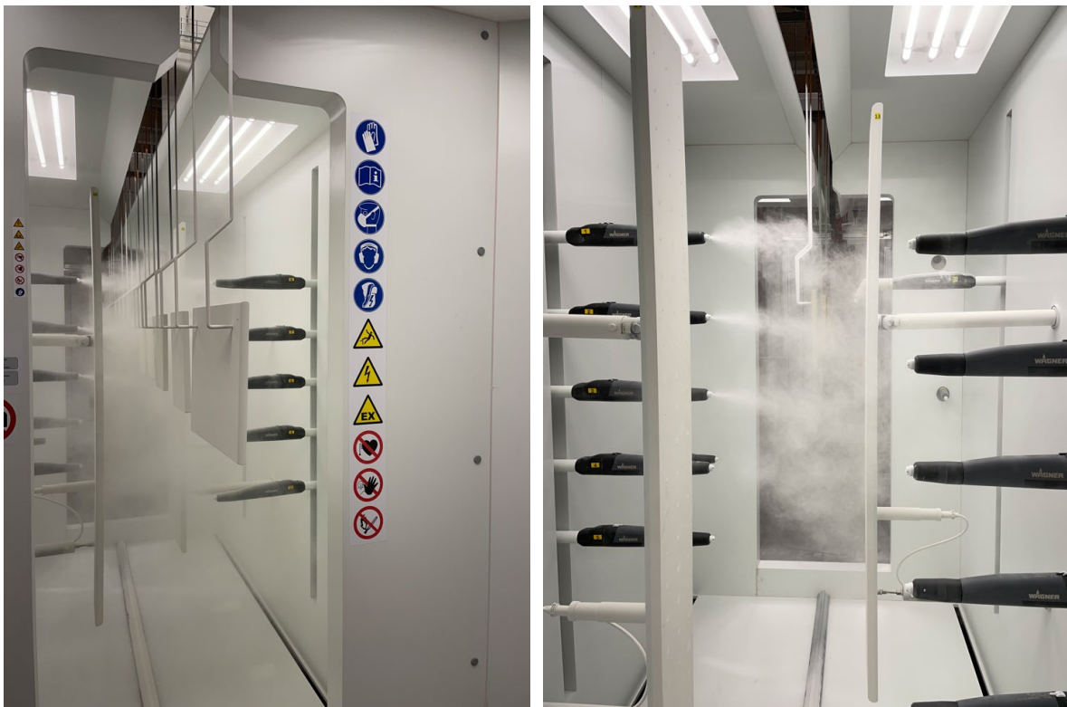
Powder coating of non-metallic workpieces in the M-Cube booth with support of Field Controllers
