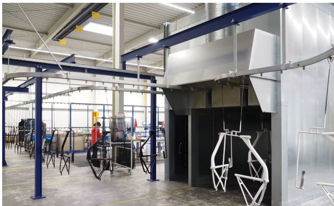
After applying the paint and passing through the oven and cooling zone (right), the frames receive their decors (center) and pass through the process a second time for the application of the clear lacquer.
