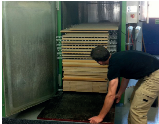
Forced conditioning of MDF boards in a conditioning room to a moisture content from 4.5 % to 6.5 % for 8 hours
