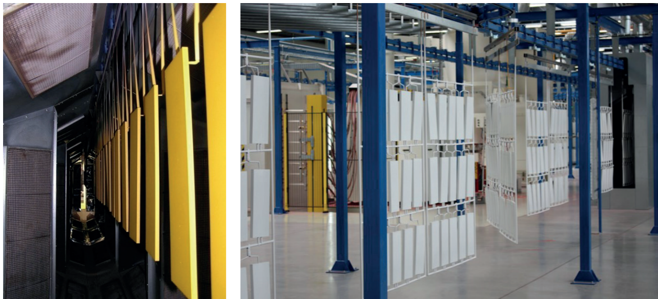
Jelling and curing by infrared radiation Left picture: Gas-catalytic IR oven / Right picture: Cured MDF parts
