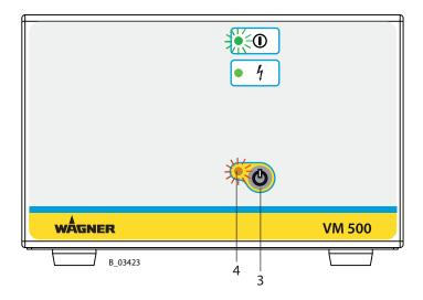
If you want to spray without high-voltage, select the standby mode. Press push button (3) briefly and the "Standby" illuminated display (4) lights up.
