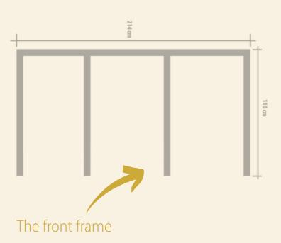
Repeat the previous steps to assemble the front frame using the already trimmed beams.
