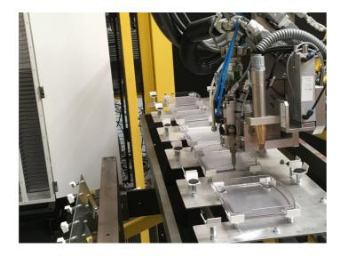
The British manufacturer **ASD Lighting** has been producing a wide range of lights for various applications since 1983. In order to keep the promise of "delivery in one week", the sealing process is now carried out in-house. The highprecision **ContiFoam foam dosing technology from Reinhardt-Technik GmbH** (member of the WAGNER Group) selected for this ensures high production quality at reduced costs.
