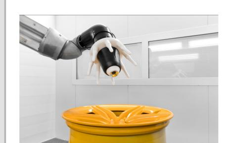
The TOPFINISH Bell 1S and RobotBell 1 highspeed rotation atomizers are equally well suited as all-round units for water- and solvent-based coatings. Both models are now also available as variants with external charging, especially for use with water-based coatings. This not only gives you efficient results, but can also reduce system costs for water-based coating applications.
