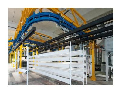
The Italian company SPRECH has installed a powder coating system for its metal canopies. The result: "Within one working day, we are able to change fifteen to twenty different colors in just 6 minutes and with one operator. Since the start-up, we have already recorded significant powder savings, thanks to a 90% overspray recovery rate."
