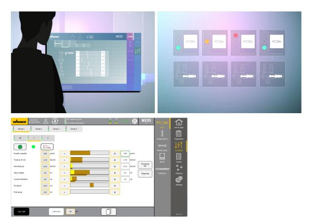
The status of each individual gun or injector is clearly displayed on the touchscreen in a traffic light system. The request for the next wear part change only appears when it is actually necessary.
