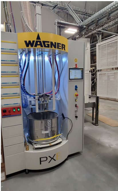
Compact PXE powder center for efficient powder feeding from the fluid container or powder box
