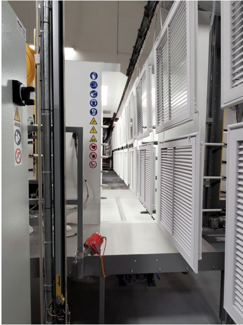
Automatic coating of metal casings for air outlets and heating coils
