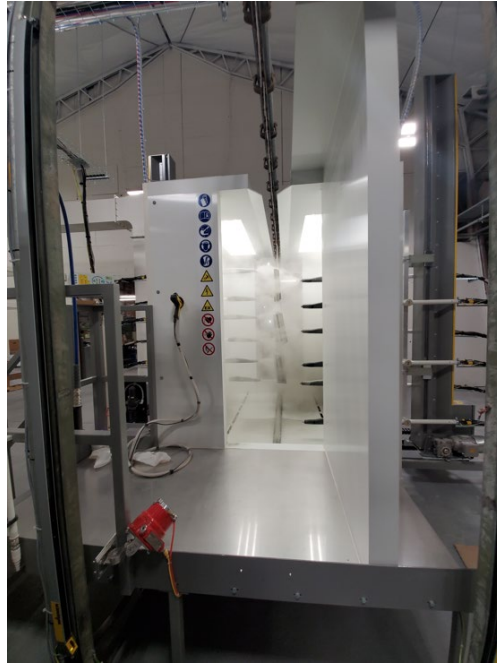
Automatic coating of metal casings for air outlets and heating coils
