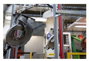
By means of a laser scan, the workpiece contours are recorded before powder coating. The gun distances in the booth are optimized accordingly by the automatic gap, height and depth control.
