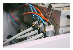
WAGNER's injector technology enables low-air powder feeding with high coating efficiency.
